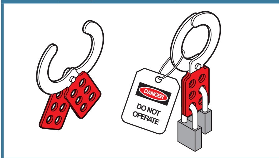
FIGURE 3: Example of tag and lockout with the padlocks of two workers.
