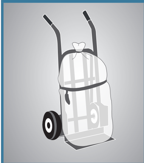
FIGURE 32 A trolley can eliminate many of the risks involved in manual handling, however, the load will still need to be manoeuvred onto the trolley and through the workplace.
