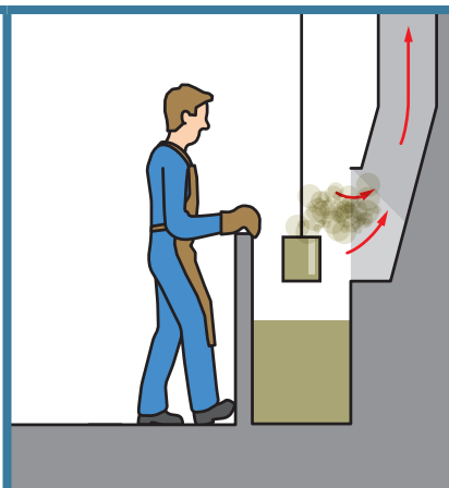
DIAGRAM 2: Side hood ventilation for an open surface tank
