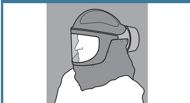
FIGURE 7: Powered, air-purifying, ventilated respirator.
