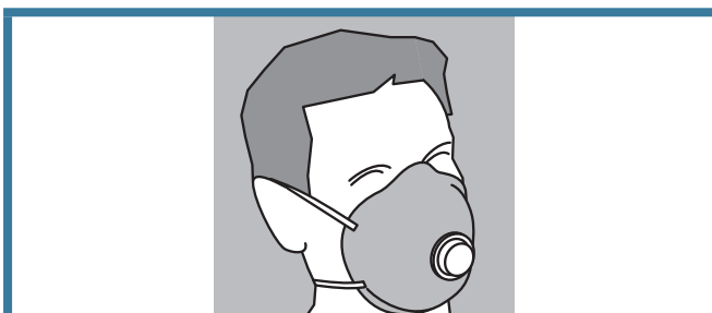
FIGURE 5: Disposable, half-face particulate respirator.
