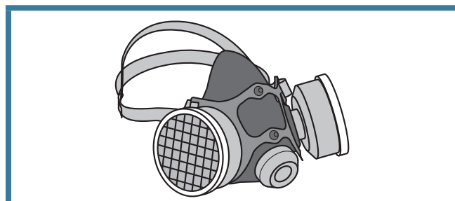
FIGURE 6: Half-face, particulate filter (cartridge) respirator.
