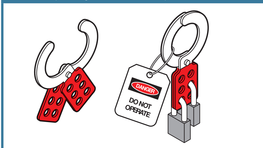
FIGURE 3: Example of tag and lockout with the padlocks of two workers.
