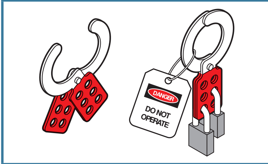
FIGURE 9 Example of lock-out with a tag and the padlocks of two workers
