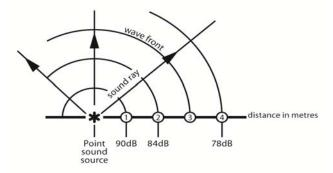
If a small sound source produces a sound level of 90 dB(A) at a distance of 1 metre, the sound level at 2 metres distance is 84 dB(A), and at 4 metres is 78 dB(A), etc.
