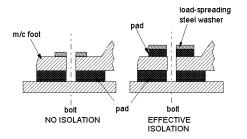
There are many types of off-the-shelf anti-vibration mounts available, for instance rubber/neoprene or spring types. The type of isolator that is most appropriate will depend on, among other factors, the mass of the plant and the frequency of vibration to be isolated. Any supplier of anti-vibration mounts will be able to advise you on this.
