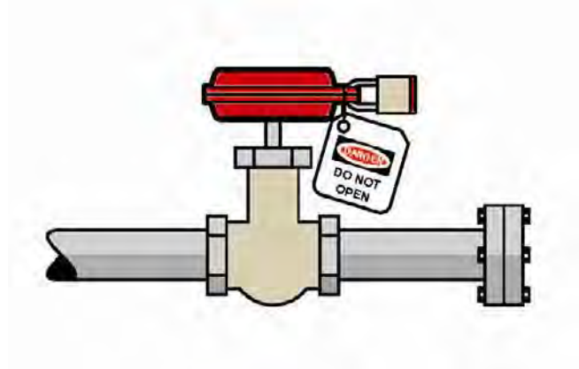
Figure 4: Open end of pipe capped. Nearest valve closed locked and tagged.
