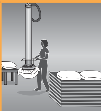
FIGURE 31: A vacuum operated lifting device can reduce the forces, awkward postures, and movements required to manually load products onto pallets.
