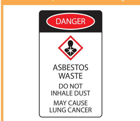
LABEL 1: Sample asbestos waste bag.
