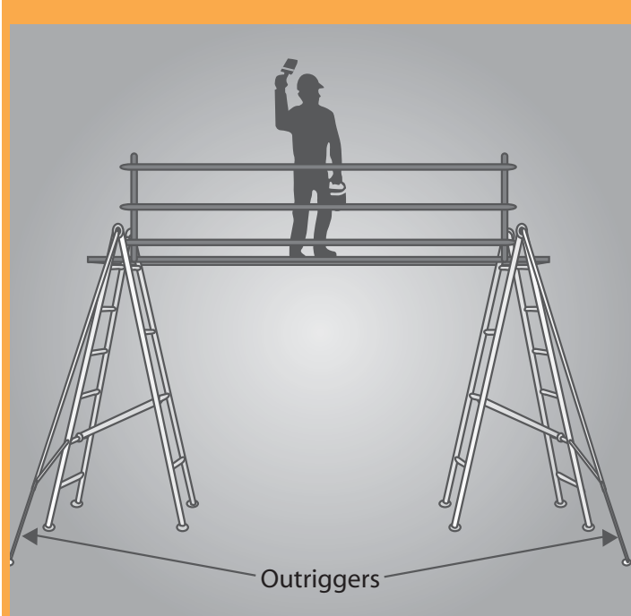
FIGURE 16: Trestle ladder scaffold with guard rails and outriggers for stability.
