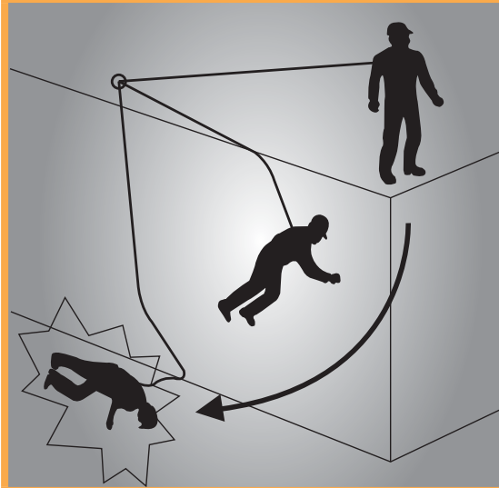
FIGURE 23: During 'swing down' the length of the lanyard and positioning of the anchor allow contact with the ground.
