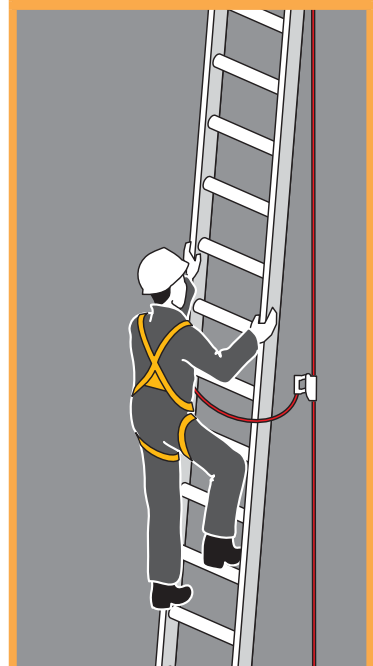
FIGURE 25: With the use of an anchorage line system, the person climbing has continuous fall protection by being attached to the anchorage line and harness.
