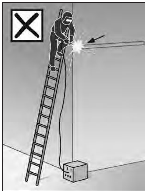
Performing hot work from a ladder
