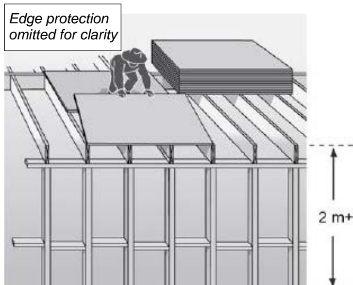
Figure 9: Laying sheet flooring at upper level
