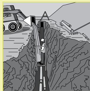
Figure 24: Example of an unguarded trench.
